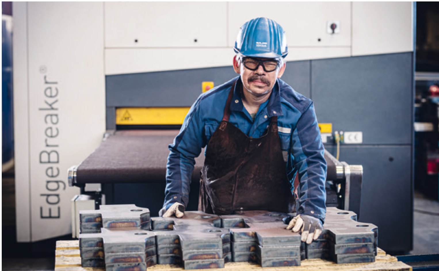
Consistent quality instead of hard labor with angle grinders: The EdgeBreaker® 4000 has vastly simplified deburring heavy plates at the steel processing specialist SÜDSTAHL. At the same time, productivity has seen a significant boost.
