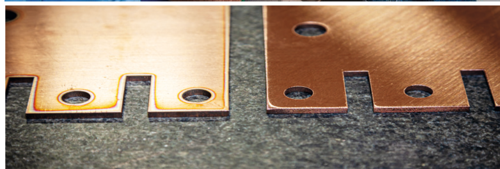
Critical edge rounding: the part after processing (on the right) showcases precise edge rounding all the way around.
