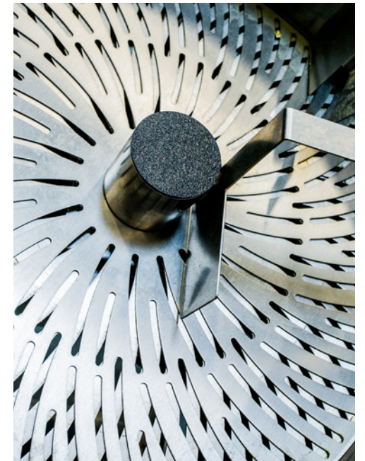
A close up of the perfectly leveled cutting blades in the final trimmer.
