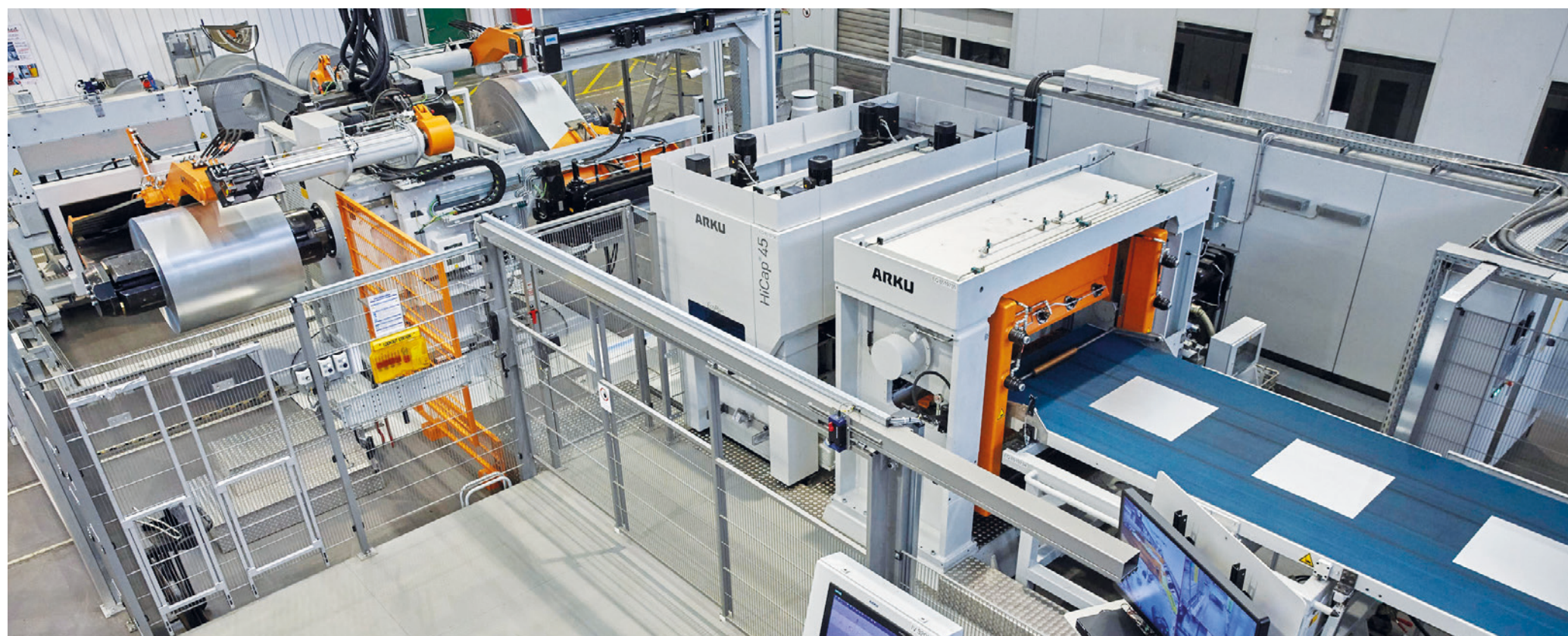
An ARKU feeding line user in the HVAC technology sector needed a cut-to-length line. This space-saving and error-free system makes an effective contribution to producing a diverse range of sheet metal blanks.
