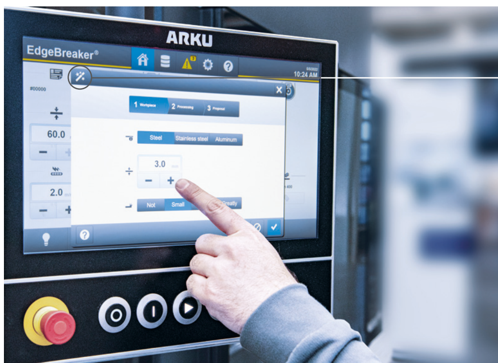
The ARKU Wizard software is now available and helps to achieve optimal deburring results by automatically configuring the deburring machines for the specific processing job.
