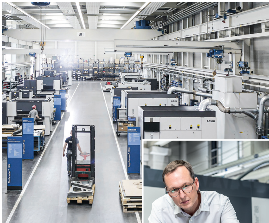
At our leveling and deburring center in Baden-Baden, we level and deburr parts and plates which are up to 2 meters wide and 50 mm thick.
