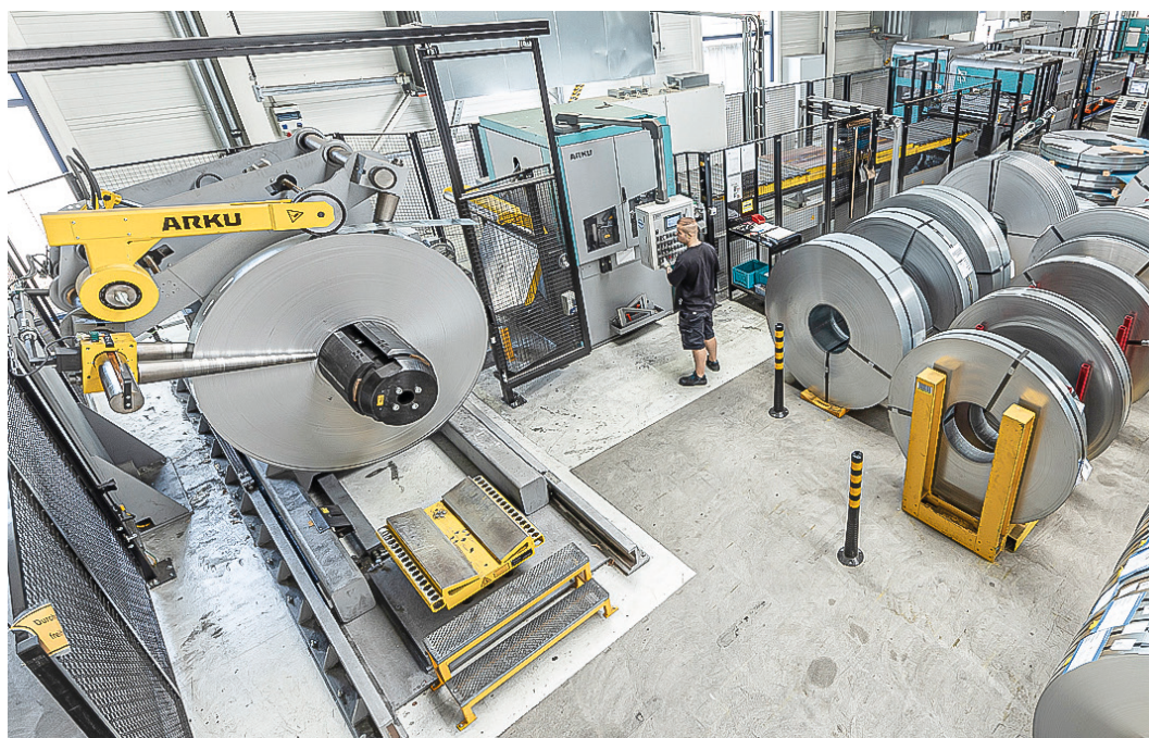
One thing is clear: With all of these coils, BITO is definitely hard at work. The ARKU coil line (left in the picture) has to prove its reliability working three shifts and with maximized capacity utilization.
