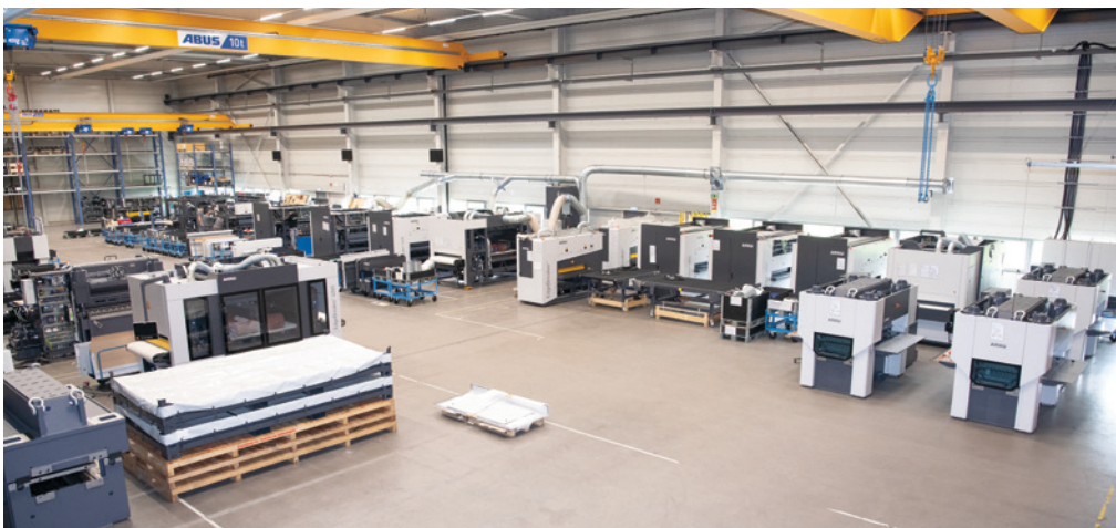
View into the production hall, where deburring machines and precision levelers are being assembled.
