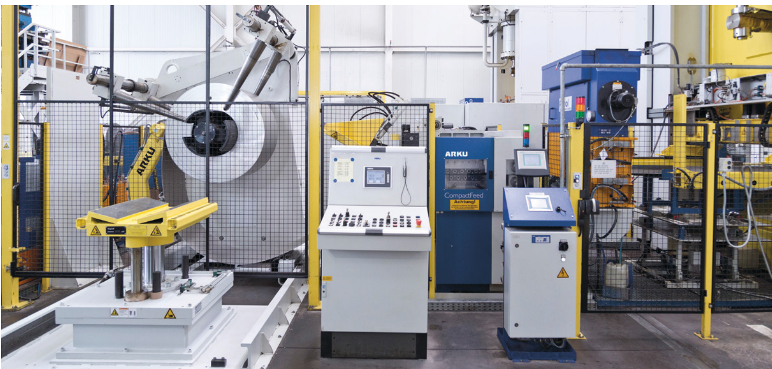
Perfectly synchronized: the combination of the press and coil feed speed is crucial for accurate stamping results without any errors.
