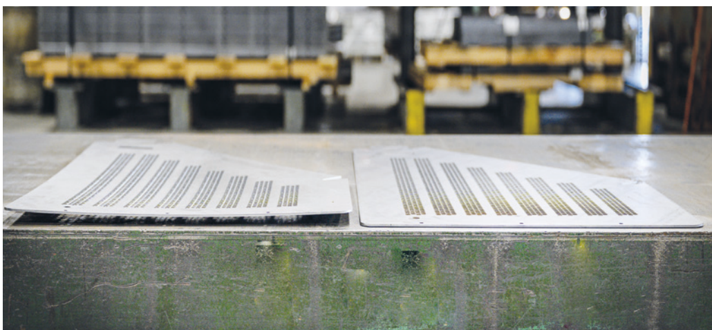
Thanks to the ARKU FlatMaster® 55, perforated laser cut parts turn flat and stress relieved in seconds.
