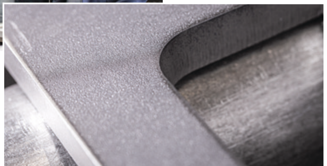
No burrs, rounded edges and flat: this is how sheet metal parts can be further processed and coated.
