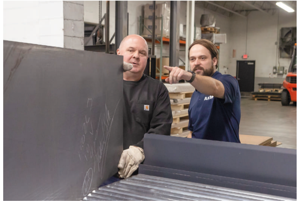
Bill Gross and Denis Weinfurter are examining a piece of metal after the leveling process to see if all flatness deformities have been removed.
