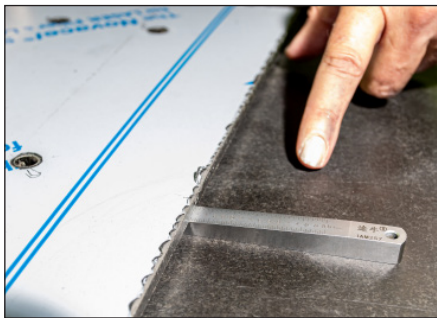
Left: Although metal sheets often appear even at first, cutting may release internal tensions, resulting in deformed products.
