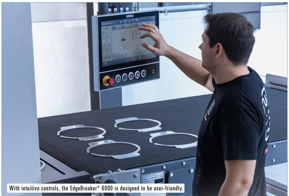
The EdgeBreaker® 6000 rapidly deburrs the materials and rounds the edges cleanly.
