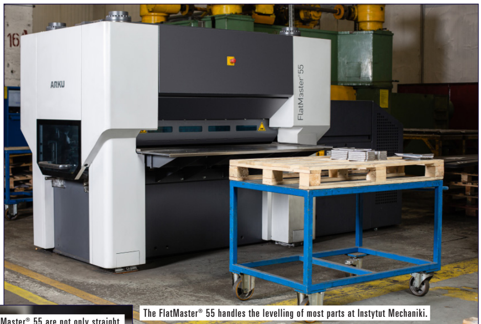
Parts levelled with the FlatMaster® 55 are not only straight, but also free of residual stresses. This makes them easier to weld.
